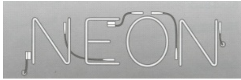
Typical Exposed Neon Installation (indoor only)
